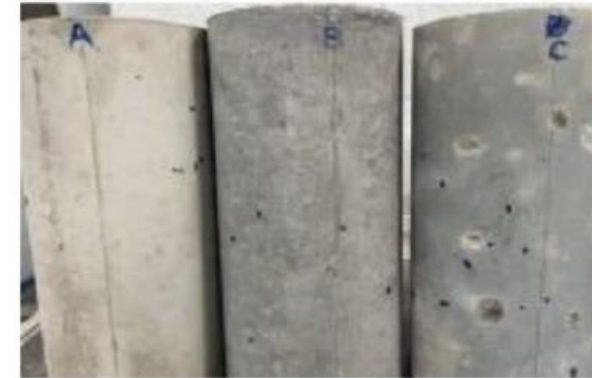
Ambiently cured and accelerated curing.
