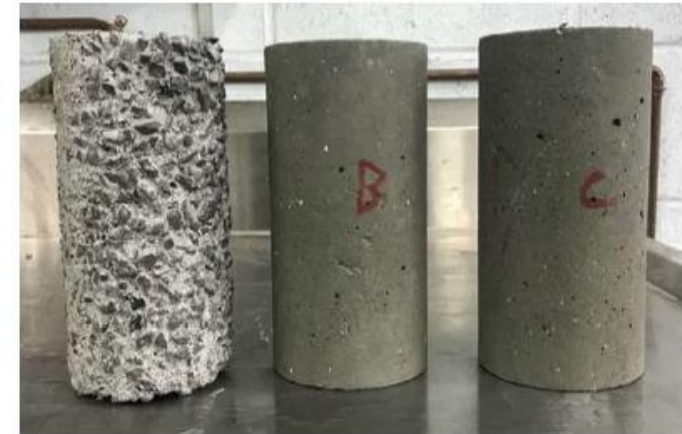
» Concrete Testing – OPC Control vs CIP Binder; Sulfuric Acid; pH 0; Temp 22°C
